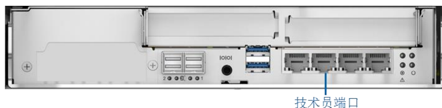
图 2-9 技术员端口位置- AS2150G2&AS2200G2&AS2600G2
